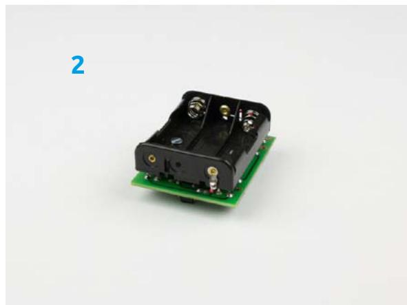
1. Solder a piece of wire (+/- 10 cm.) to the "+" pole lip of the battery holder.
