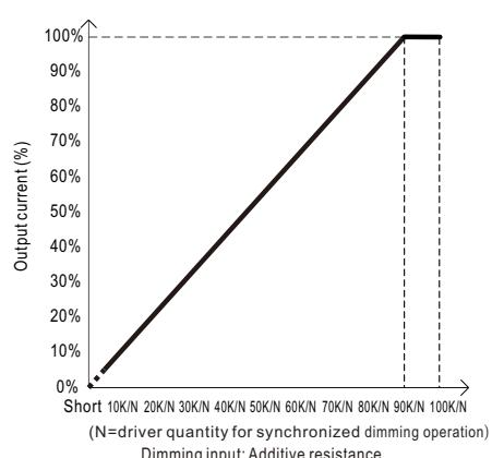
Note : 1. Min. dimming level is about 3% and the output current is not defined when 0% < Iout < 3%.
