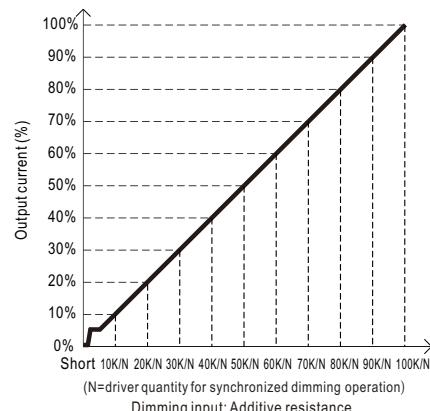
Note : 1. Min. dimming level is about 5% and the output current is not defined when 0% < Iout < 5%.
