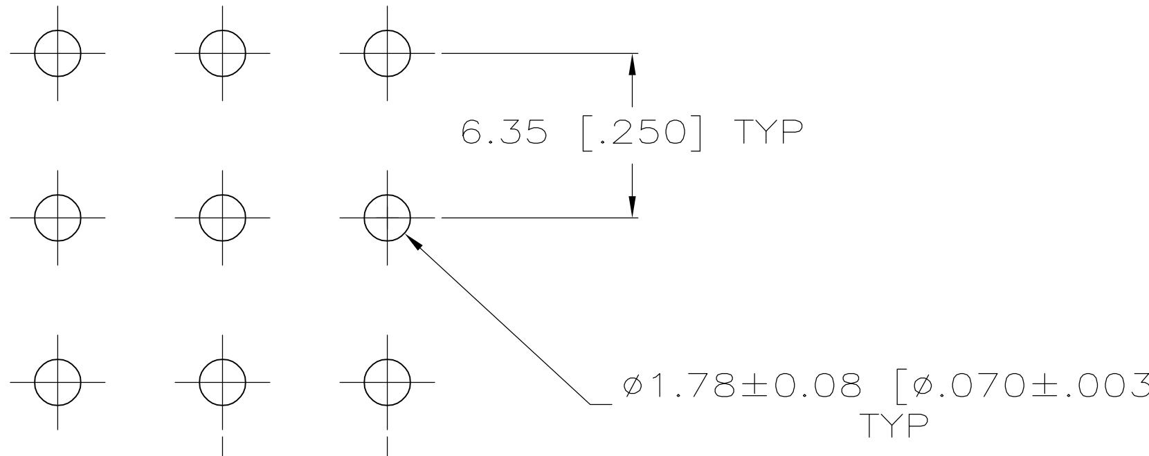
RECOMMENDED LAYOUT FOR 1.58 [.062] THICK PC BOARD
