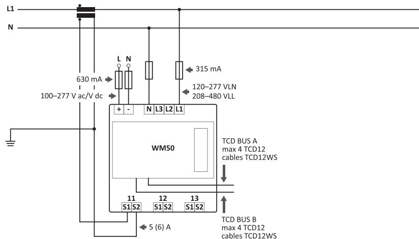
**Fig. 3 Single-phase system with neutral (2-wire)**
