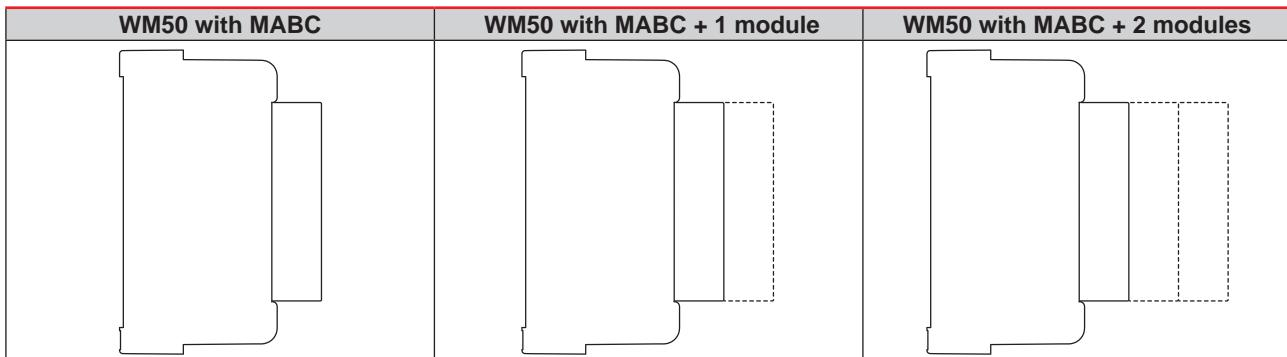
WARNING: maximum 1 module per type. A digital input/output module cannot be connected with an analog input module.
