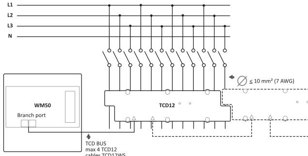
**Fig. 12** Three-phase system with neutral (4-wire).
