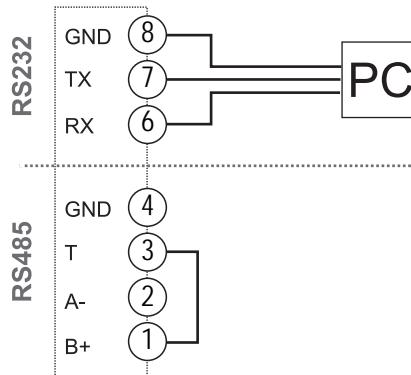
Fig. 9 M C 485232. RS232 serial port.
