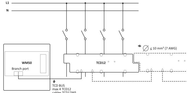
**Fig. 13** Single-phase system with neutral (2-wire)
