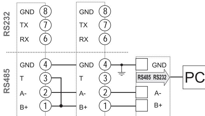
Fig. 10 M C 485232. RS485 serial port.
