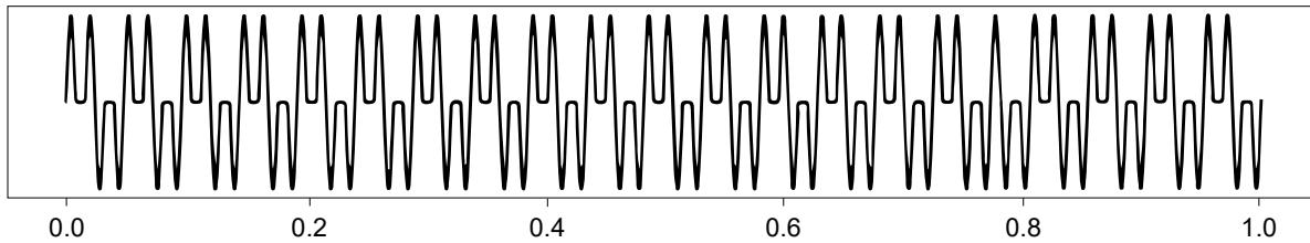
The advantage of AFC over Burst is the reduction in thermal cycling. Another advantage of AFC is that visual flicker is less noticeable than Distributed thus making it suitable for shortwave infrared heater applications.
