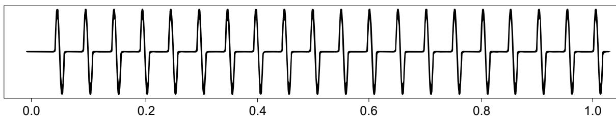
Output with Distributed firing mode @ 50% control level:
