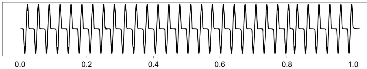
Output with Distributed firing mode @ 66% control level:
