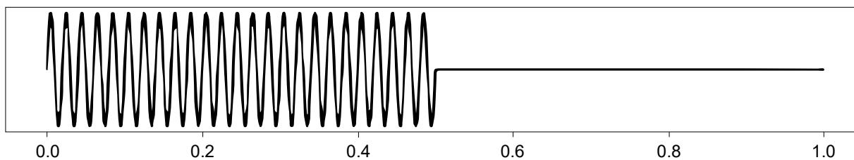
Output with Burst firing mode @ 66% control level:
