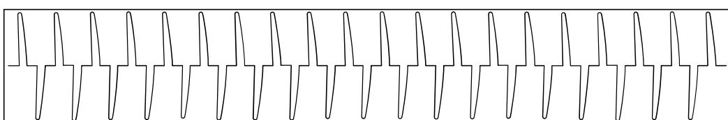
The advantage of Phase Angle over the other switching modes is its precise resolution of power. However, Phase Angle generates excessive harmonics vs other switching modes. With Phase Angle control, the flickering of IR heaters is eliminated completely.
