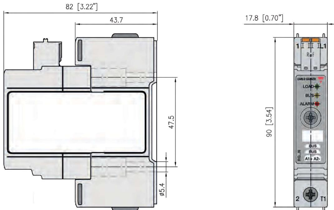
Housing width tolerance +0.5mm, -0mm as per DIN 43880.
