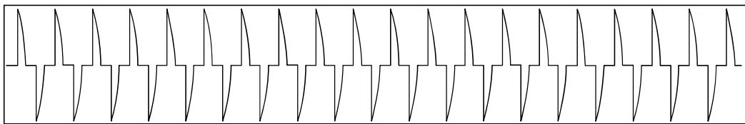
Output with Phase Angle mode @ 50% control level:
