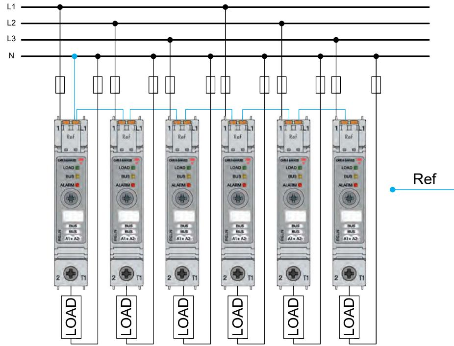
Loads connected between phases. Reference connection (Ref) should always follow the return path of the load
