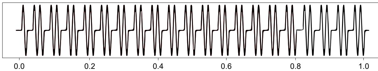
The advantage of Distributed over Burst is the reduction in thermal cycling. On the other hand, Distributed suffers from worse harmonics/emissions than Burst.
