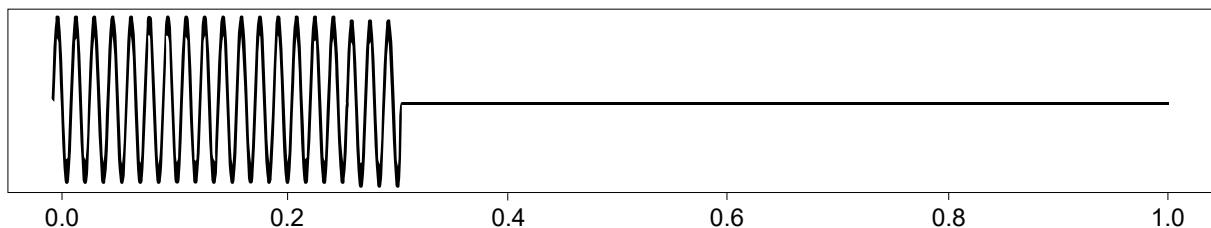
Output with Burst firing mode @ 50% control level:
