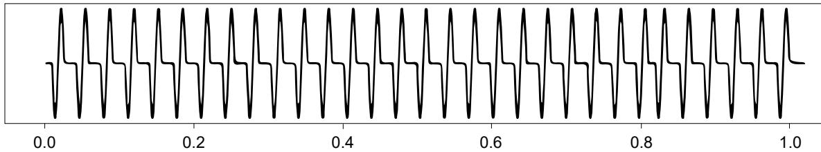
Output with Advanced full cycle firing mode @ 66% control level:
