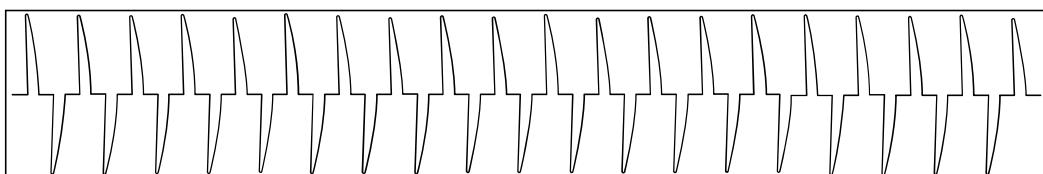
Output with Phase Angle mode @ 66% control level:
