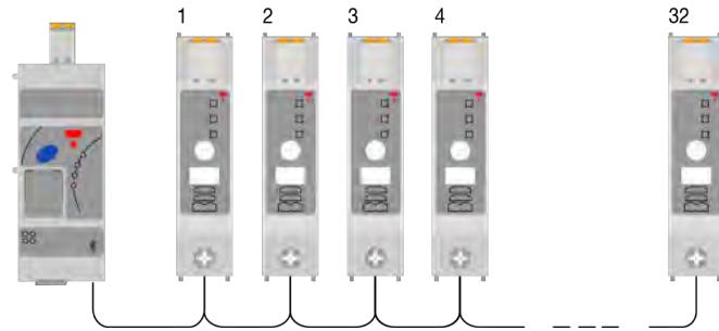
In case of an RG..N replacement, or any changes to the NRG bus chain, the RG..Ns have to be re-addressed. Follow the procedure below to re-address the RG..Ns on the NRG bus chain manually. Alternatively, auto-addressing can be done via an 'SDO' (check NRG EtherCAT User Manual for further information)
