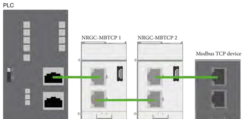
**Fig. 3 Example of a line configuration of the NRGC-MBTCP with other Modbus TCP devices and controller**
