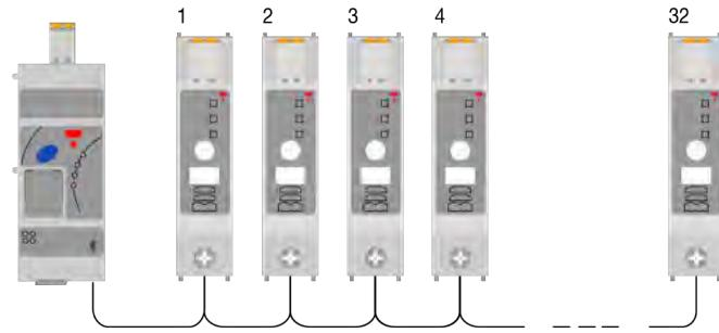
In case of an RG..N replacement, or any changes to the NRG bus chain, the RG..Ns have to be re-addressed. Follow the procedure below to re-address the RG..Ns on the NRG bus chain manually. Alternatively, auto-addressing can be done via communication. (check NRG Modbus TCP User Manual for further information)
