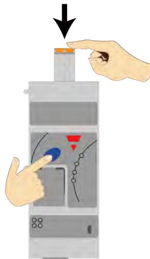
**Fig. 1** Hold the blue button while powering up the NRGC-MBTCP
