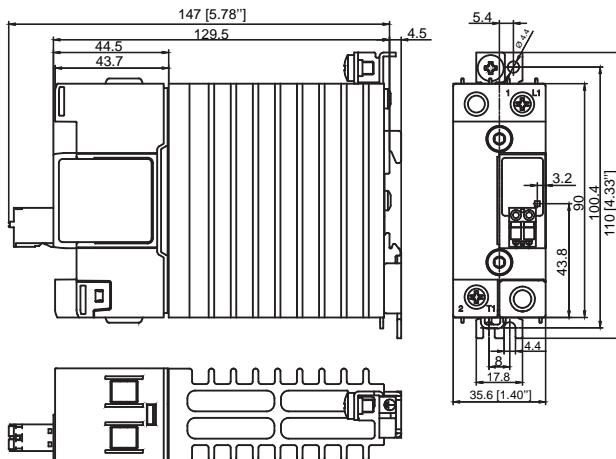
Housing width tolerance +0.5mm, -0mm as per DIN 43880. All other tolerances +/- 0.5mm.
