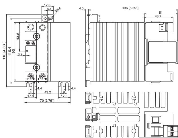
Housing width tolerance +0.5mm, -0mm as per DIN 43880. All other tolerances +/- 0.5mm.
