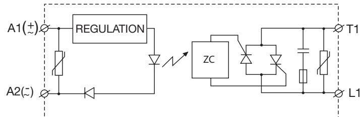
Note: Varistor on output is not included in the RGH1A69...models
