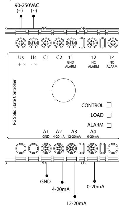
Note: Control input shall be connected either to A1-A2 or A1-A3 or A1-A4 only
