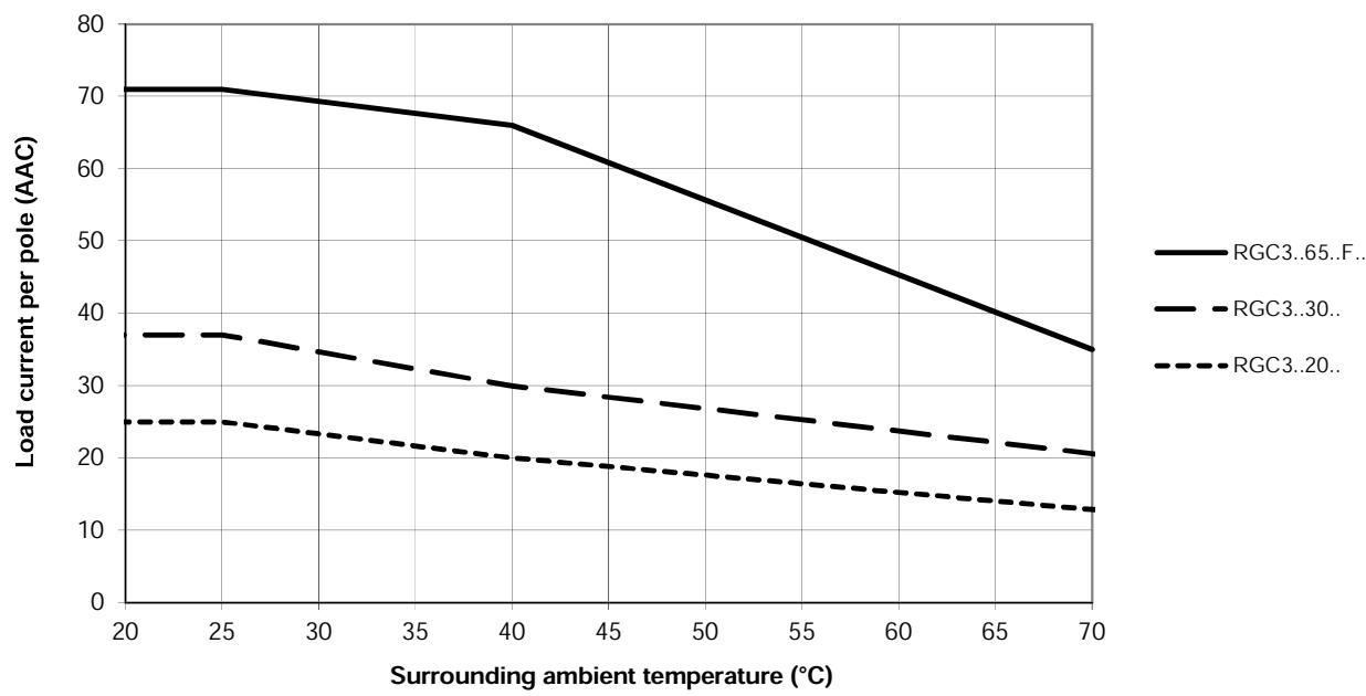
Note: Versions that utilise 24 VAC external supply (Us) are limited to a maximum operating temperature of 60°C (140°F)
