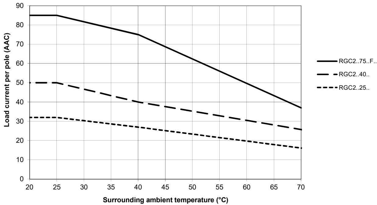
Note: Versions that utilise 24 VAC external supply (Us) are limited to a maximum operating temperature of 60°C (140°F)
