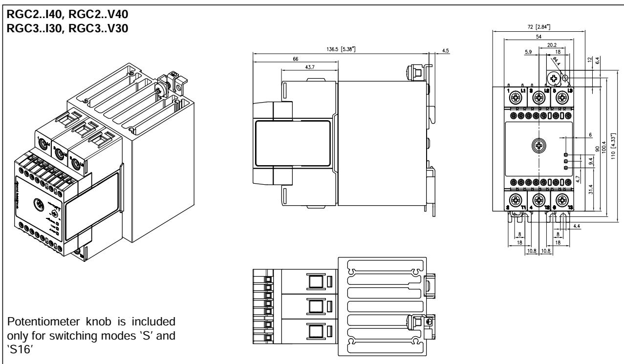
Housing width tolerance +0.5mm, -0mm as per DIN 43880. All other tolerances +/- 0.5mm.
