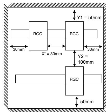
\* Refer to Current Derating curves at 0mm for 0mm spacing between units
