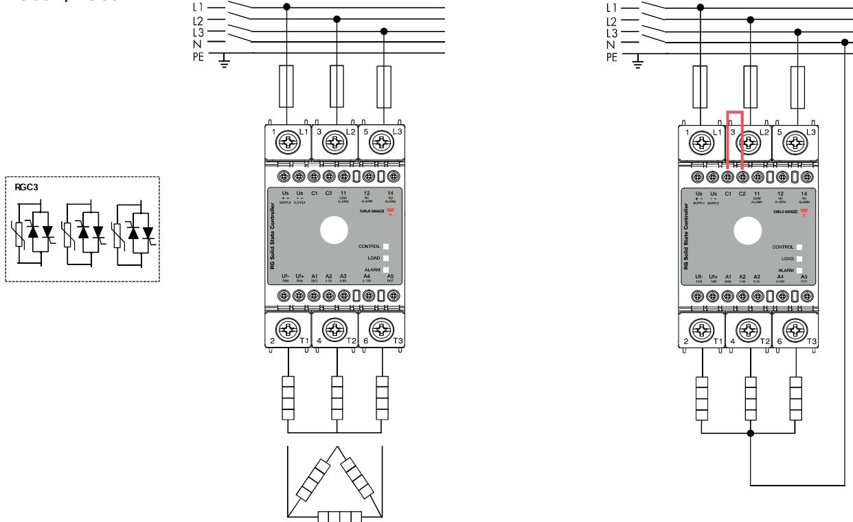
Note: Short link external connection is required between C1 and C2 terminals for 4-wire 3-phase systems.
