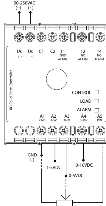
Note: Control input shall be connected either to A1-A2 or A1-A3 or A1-A4 or A1-A3-A5 in case an external potentiometer is used.
