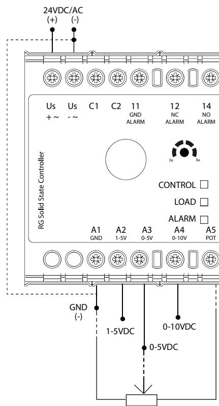
Note: Control input shall be connected to terminals A1-A4 in the case of the RGC3P..S.. In the case of the RGC3P..S16.. the control input shall be connected to either A1-A2 or A1-A3 or A1-A4 or A1-A3-A5 in case an external potentiometer is used.
