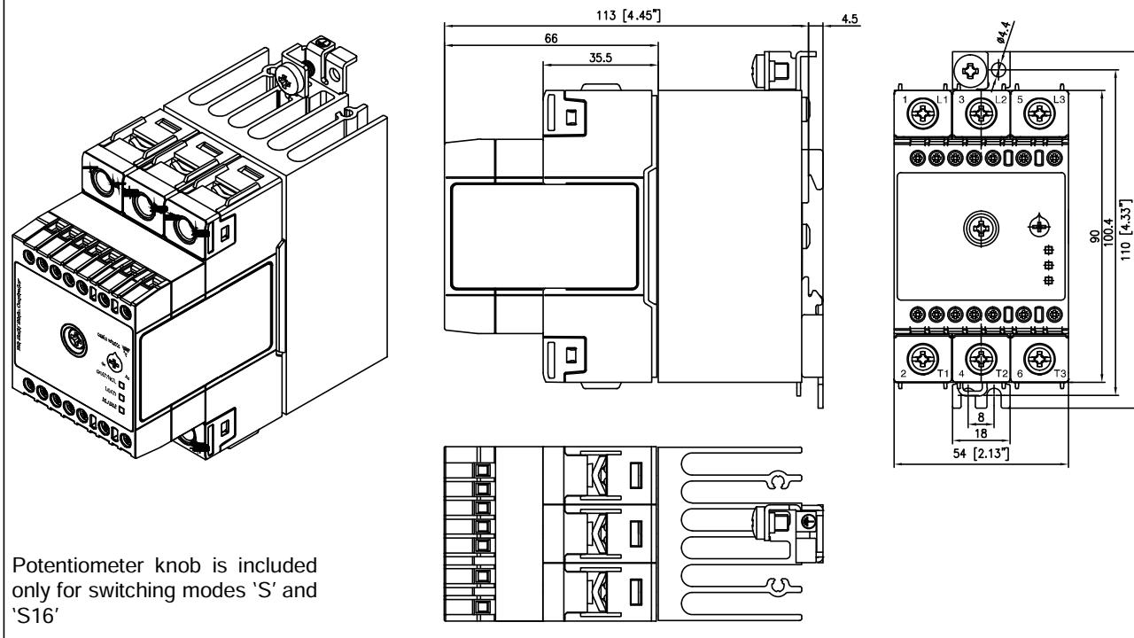
Housing width tolerance +0.5mm, -0mm as per DIN 43880. All other tolerances +/- 0.5mm.
