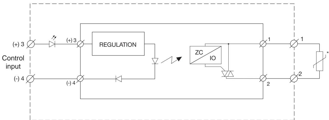
\* The varistor is not included in the solid state relay. Connecting a varistor across terminals 1-2 helps protect the solid state relay against damages by over-voltage.
