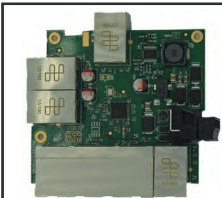
Embedded format, takes up minimal space, with mounting holes are connected to Functional Earth
