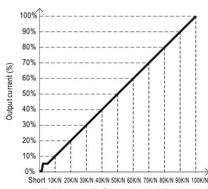
Note : 1. Min. dimming level is about 8% and the output current is not defined when  $0\% < \text{Iout} < 8\%$ .
