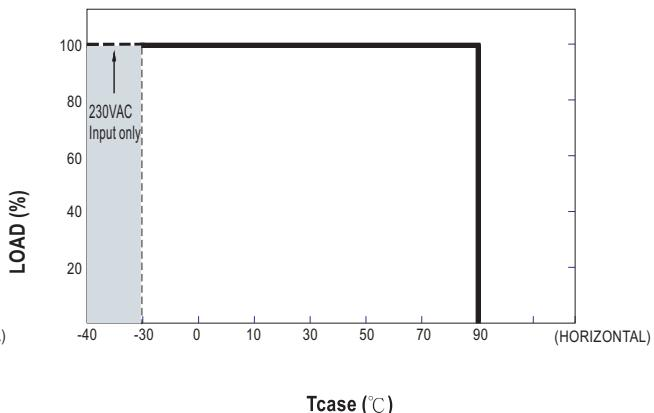
If XLG-100 operates in Constant Current mode with the rated current the maximum workable  $T_a$  is  $60^{\circ}\text{C}$  (Typ. 230VAC) or  $50^{\circ}\text{C}$  (Typ. 100VAC)
