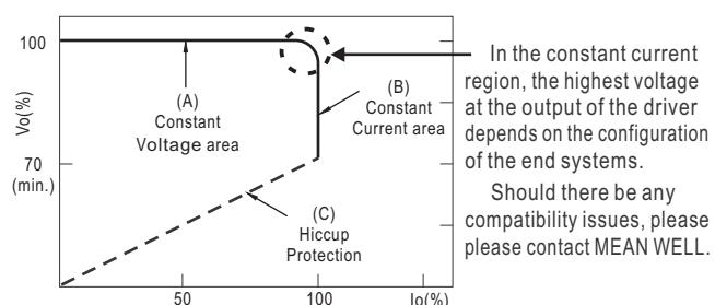
Typical output current normalized by rated current (%)
