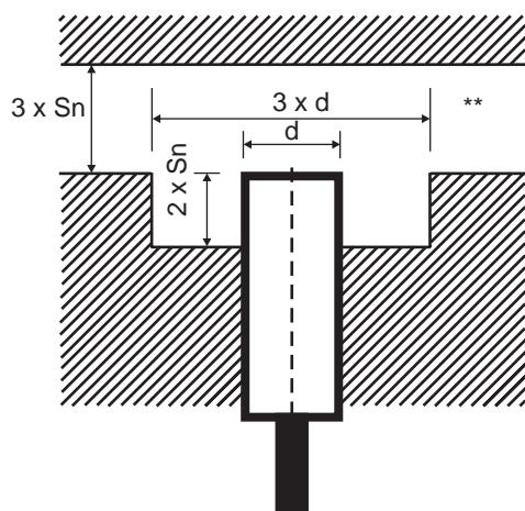
**Fig. 27** Non-flush sensor, when installed in damping material
