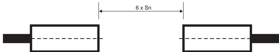
**Fig. 29** For sensors installed opposite each other, a minimum space of  $6 \times S_n$  (the nominal sensing distance) must be observed
