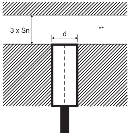
**Fig. 25** Flush sensor, when installed in damping material
