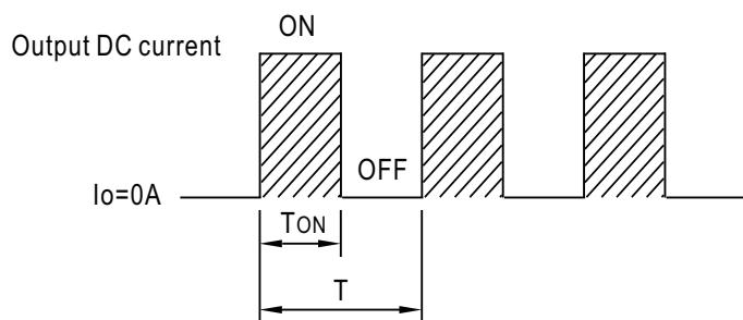
$$\text{Duty cycle(%)} = \frac{\text{TON}}{\text{T}} \times 100\%$$
