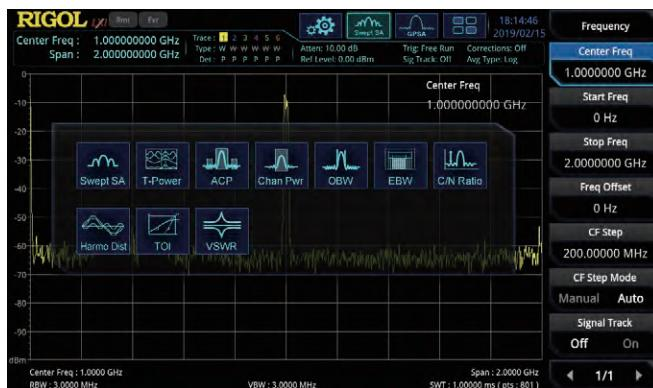
Advanced measurement mode provides test items required for the transmitter test such as multichannel power, ACP, and occupied BW.
