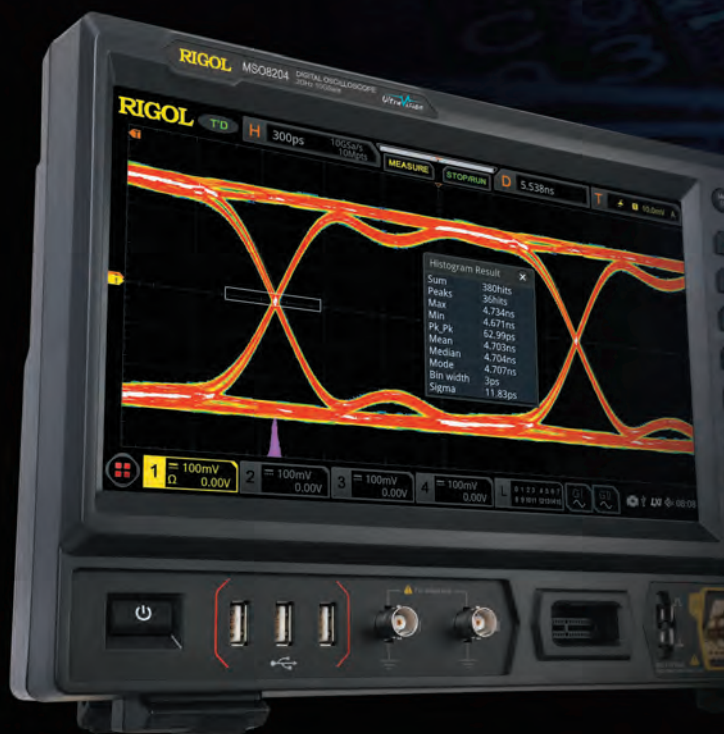
Perform eye measurement on the 622 Mb/s signal.
