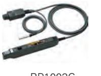
RP1003C   | Current Probe                   | BW: DC to 50 MHz<br>Max. input<br>AC P-P: 50 A (noncontinuous),<br>AC RMS: 30 A<br>Compatibility: all <b>RIGOL</b> scopes.<br>Must order RP1000P power supply.                                      |
