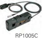
RP1005C | Current Probe                   | BW: DC to 10 MHz<br>Max. input<br>AC P-P: 300 A (noncontinuous), 500 A (@pulse width $\leq 30$ us),<br>AC RMS: 150 A<br>Compatibility: all <b>RIGOL</b> scopes.<br>Must order RP1000P power supply. |
