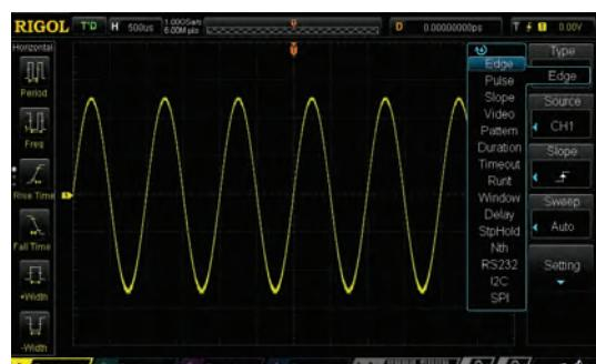
Built-in dual-channel 25 MHz source (DS1XX4Z-S Plus)
