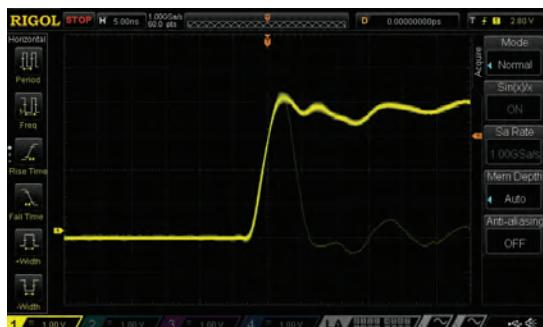
UltraVision: waveform recording and playback functions
