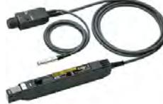
RP1003C   | Current Probe | <ul style="list-style-type: none"> <li>• BW: DC~50 MHz</li> <li>• Maximum Input AC P-P: 50 A (non-continuous)</li> <li>• AC RMS: 30 A</li> <li>• Compatibility: All models of RIGOL's digital oscilloscopes</li> <li>• Required to order RP1000P power supply.</li> </ul>                                                 |
