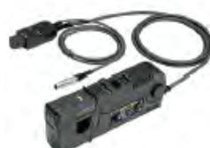
RP1006C | Current Probe | <ul style="list-style-type: none"> <li>• BW: DC~2 MHz</li> <li>• Maximum Input AC P-P: 700 A peaks, non-continuous</li> <li>• AC RMS: 500 A</li> <li>• Compatibility: All models of RIGOL's digital oscilloscopes</li> <li>• Required to order RP1000P power supply.</li> </ul>                                           |
