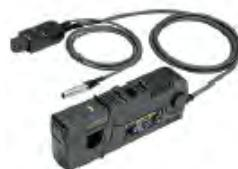
RP1005C | Current Probe | <ul style="list-style-type: none"> <li>• BW: DC~10 MHz</li> <li>• Maximum Input AC P-P: 300 A (non-continuous), 500 A (@pulse width <math>\leq 30</math> us)</li> <li>• AC RMS: 150 A</li> <li>• Compatibility: All models of RIGOL's digital oscilloscopes</li> <li>• Required to order RP1000P power supply.</li> </ul> |
