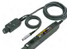
RP1004C  | Current Probe | <ul style="list-style-type: none"> <li>• BW: DC~100 MHz</li> <li>• Maximum Input AC P-P: 50 A (non-continuous)</li> <li>• AC RMS: 30 A</li> <li>• Compatibility: All models of RIGOL's digital oscilloscopes</li> <li>• Required to order RP1000P power supply.</li> </ul>                                                |
