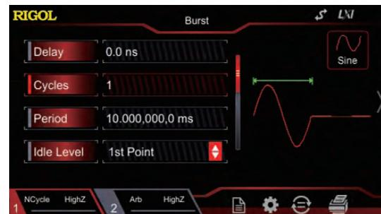
Various analog and digital modulation functions
