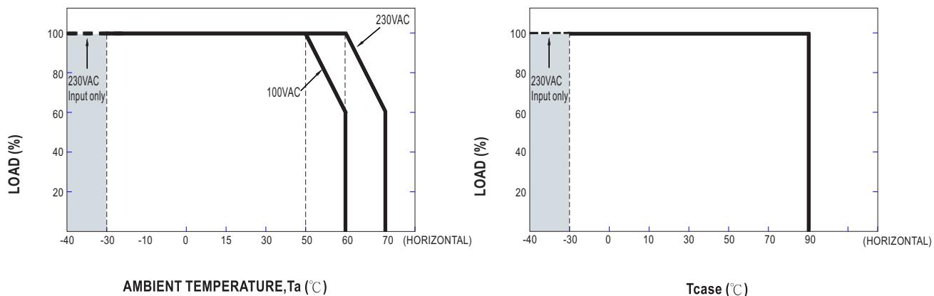
Note: 1. If XLG-75-DA2 operates in Constant Current mode with the rated current the maximum workable Ta is 60°C (Typ. 230VAC) or 50°C (Typ. 100VAC)
