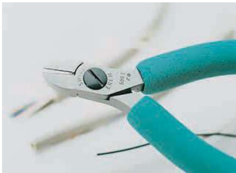
The 599TFO has wear resistant tungsten carbide cutting edges and all round capability. It is able to cut Vectran™ braided wires, fibre optics, Kevlar® and small stainless steel braids and wires.
