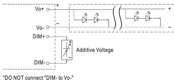
**※ Smart timer dimming function (for Dxx-Type by User definition)**
