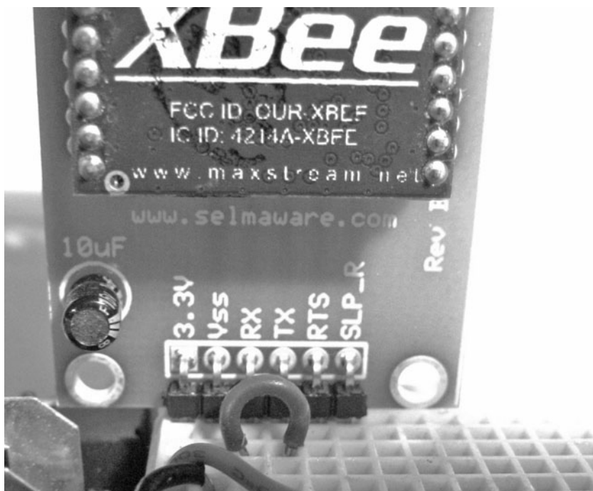
Figure 5-8 Remote XBee connections for loop-back.
