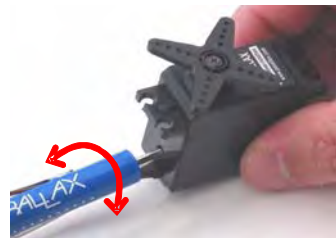
Gently turn screwdriver to adjust potentiometer
