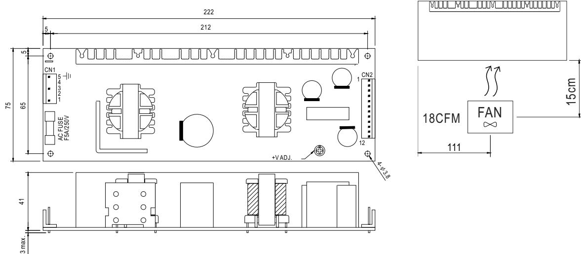
AC Input Connector (CN1) : JST B5P-VH or equivalent
