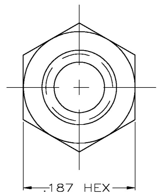
△ COLD ROLLED STEEL PER ASTM A108.
