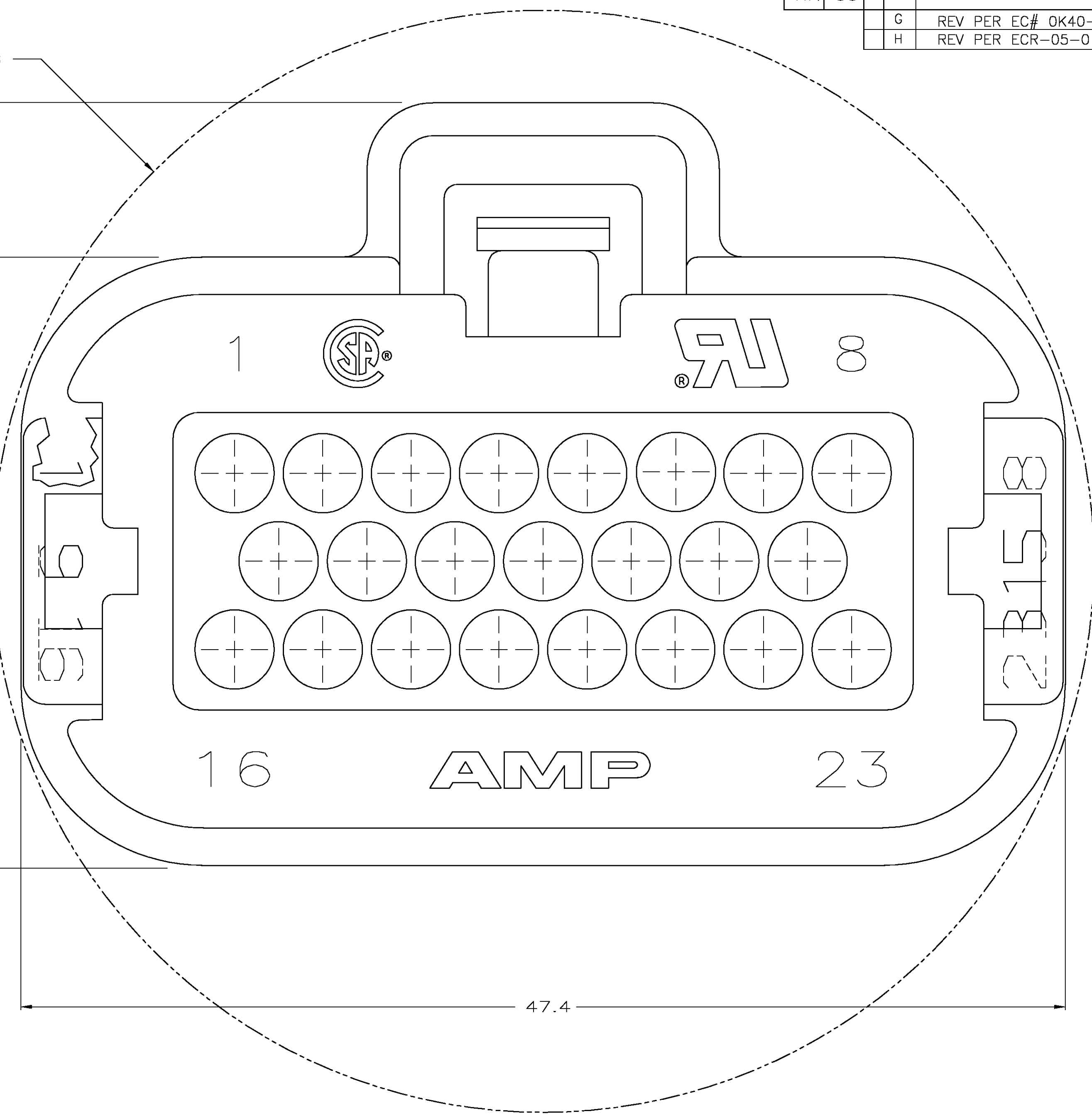
⚠ HOUSING COLORS ARE MECHANICALLY KEYED TO MATE ONLY WITH IDENTICALLY COLORED HEADER ASSEMBLIES. ⚠ OPTIONAL CONSTRUCTION OF LATCH OVERSTRESS FEATURE.
