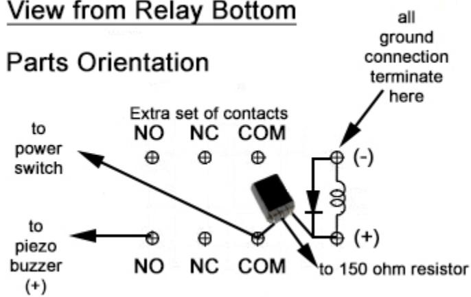
That loop at the end, will hold all the negative wires that will need to be joined: from the sensor, the battery and the piezo buzzer.
