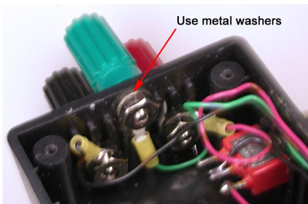
Note that we threw away the plastic washers and used metal washers instead so that the ring terminals were properly seated and connected.
