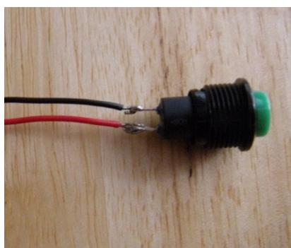
Attach two pieces of wire to the button and solder them into place. Strip the ends about 2-3mm long and tin them with solder.
