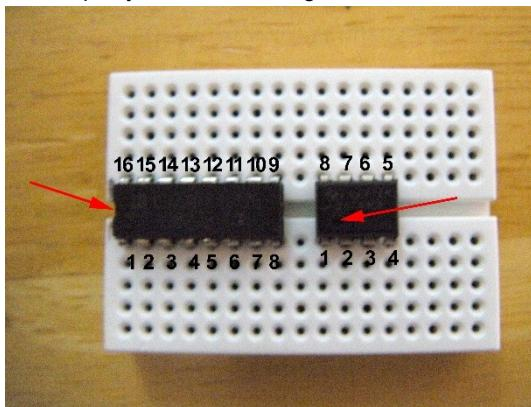
Plugged in, they now should look exactly like the photo on the left. The small IC, the 741 op-amp, will have a dot showing pin one, and have the dot facing the same direction as the 4017 chip as shown at right by the red arrows.
