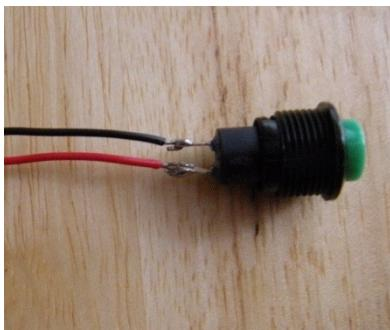
Attach two pieces of wire to the button and solder them into place. Strip the ends about 4-mm long. While you have the soldering iron hot, tin the ends of the wires of the 9-volt battery holder because they use stranded wire (not good for breadboards). Then, starting with smaller bits, eventually use a 7/16" drill bit to drill out a hole for the button.
