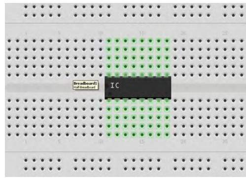
Note how each hole is connected by the colored lines representing how each hole is connected to the hole next to it in a strip called a buss.
