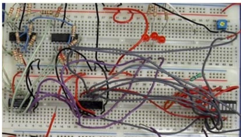
As you can see, using good wiring techniques can help keep the work organized and tracked. Having neat wiring also helps when the project does not work and needs troubleshooting.
