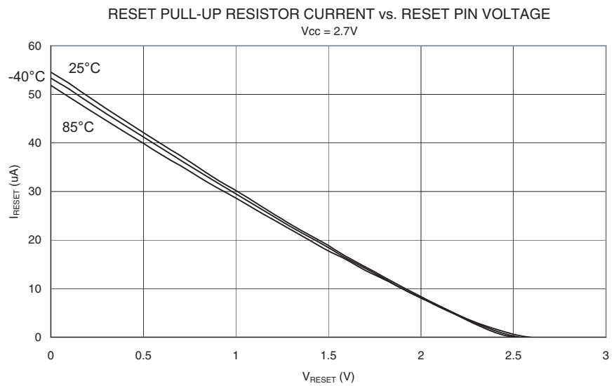
Figure 177. Reset Pull-Up Resistor Current vs. Reset Pin Voltage ( V_{CC} = 2.7V )
