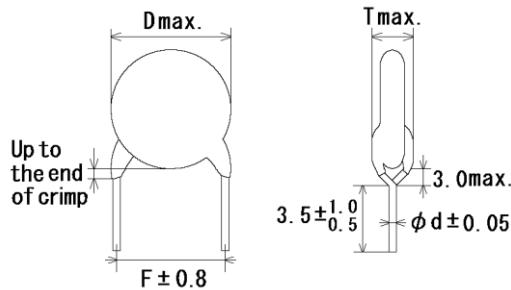
Note) The mark '\*' of Lead Style differ from lead spacing (F) and lead diameter (d).
