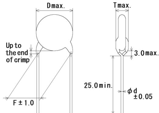
Note) The mark '\*' of Lead Style differ from lead spacing (F) and lead diameter (d).
