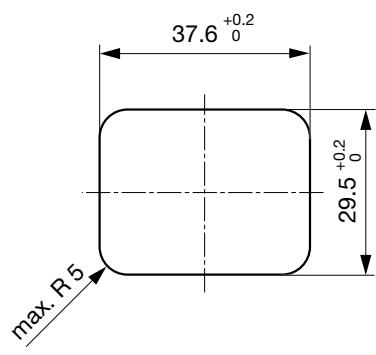
Version "along" (wires along to pin axis)
