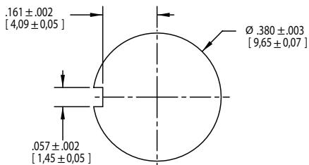
**DIMENSIONS** in inches (and millimeters)Unless otherwise specified, standard tolerance is  $\pm .010$  (0,25)
