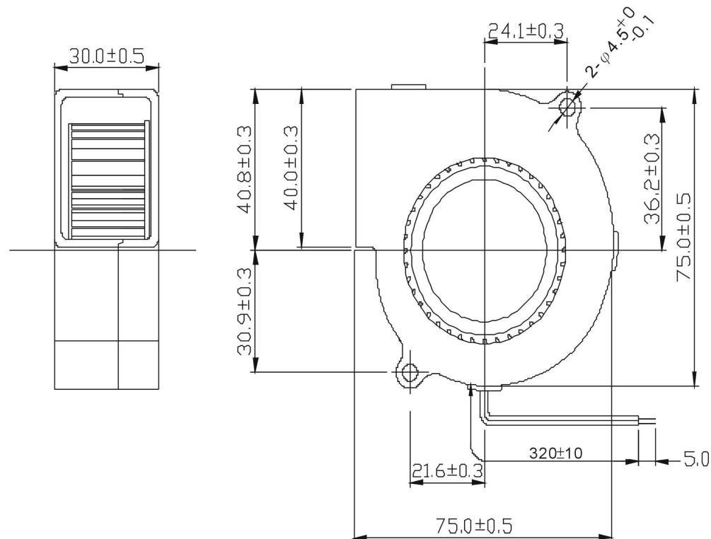
LEAD WIRES : UL 1007, AWG24 , L =  $320 \pm 10$  mm
