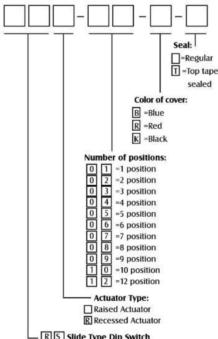
**Example:** RS-08-B-T is a slide type dip switch, raised actuator, 8 position, blue cover with top tape sealed.
