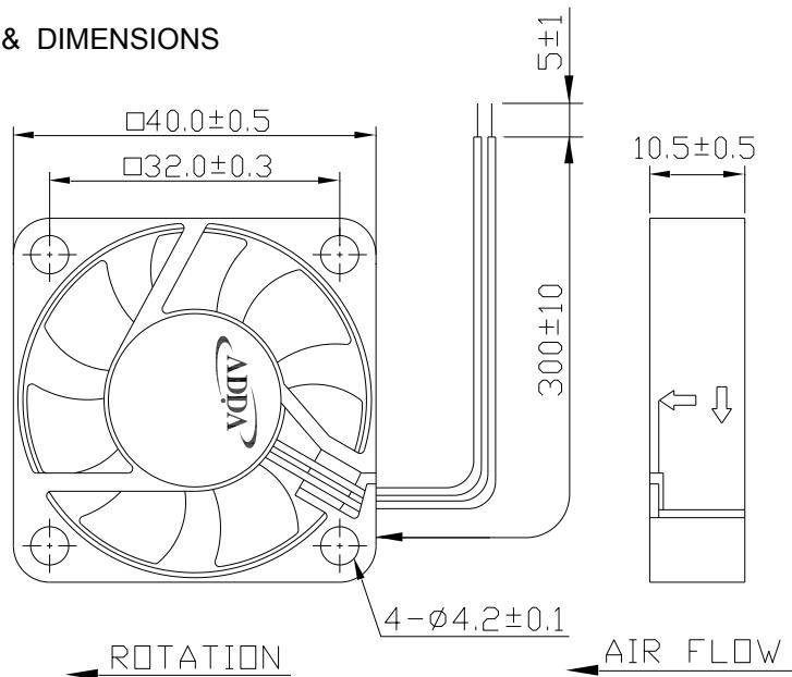
LEAD WIRES : UL 1007, AWG26, L = 300 +/- 10 mm
