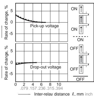
12. Actual load test (35 mA 48 V DC wire spring relay load)
