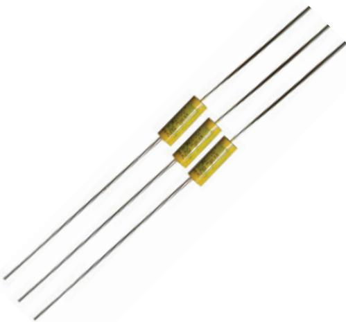
Type WMC axial-leaded polyester film/foil capacitors are ideal for automatic insertion in printed circuit boards. It is an ultraminiature version of Type WMF and the sections of these non-inductive capacitors are constructed with extended foil, polyester film, with tinned copper-clad steel leads.
