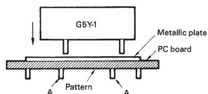
When a relay is mounted on a single-sided PC board, an isolation of only 60 to 70 dB can be obtained at 200 MHz. Therefore, to permit the relay on the single-sided PC board in a higher frequency range, a metallic plate can be inserted between the PC board and the relay, then connected to the ground pattern.
