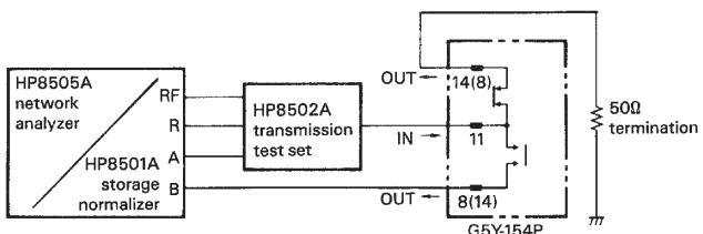
The following characteristics, when a signal is applied from input terminal 11 to output terminal 8 or from input terminal 11 to output terminal 14 of the sample, are measured with contacts unrelated to the measurement terminated at 50Ω.
