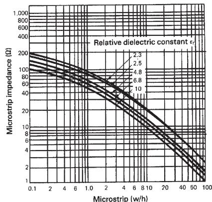
For example, when a 50Ω transmission line is to be formed using a 1.6 mm (0.06) glass epoxy type double-sided PC board, the width of the transmission line can be obtained in the following manner. Since the specific inductive capacity ( $\epsilon_r$ ) of this circuit board is 4.8,  $w/h = 1.7$  (obtained from the above table). Based on the thickness of the PC board (e.g., 1.6 mm [0.06]), the thickness of transmission line w can be calculated as follows.
