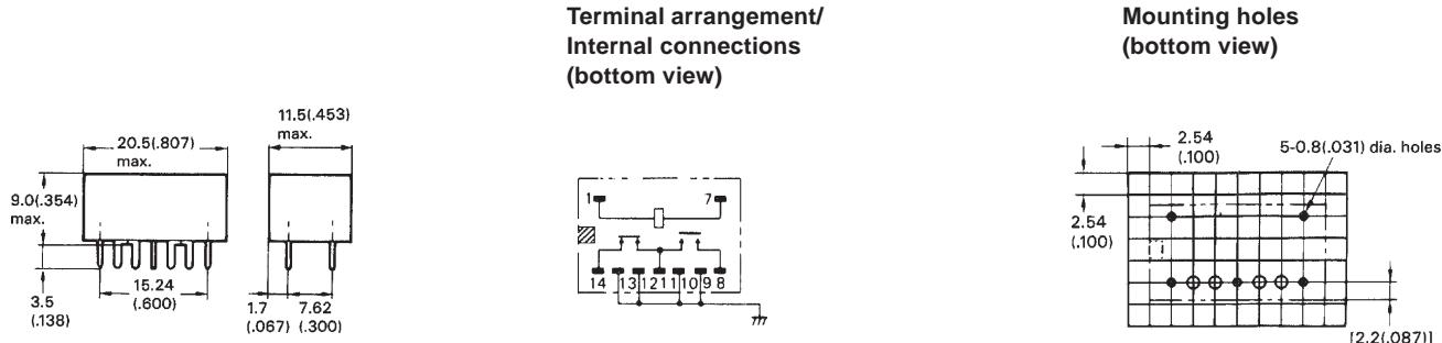
Note: Parts marked with and indicate mounting direction mark on G5Y relay.
