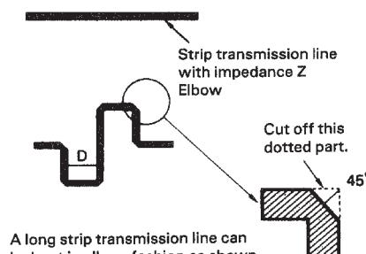
A long strip transmission line can be bent in elbow fashion as shown in the figure. The distance between the bends of the strip line (D) should be almost double the width of the strip line.
