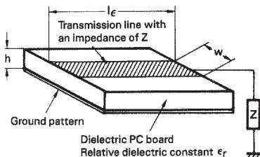
The characteristic impedance of a transmission line is determined by the type of PC board (specific inductive capacity), its thickness, and the width of the transmission line. This impedance is expressed by the following formula.
