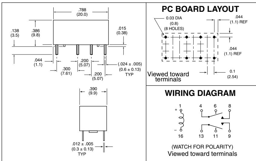
Dimensions in inches with metric equivalents in parentheses. Tolerance:  $\pm .010"$
