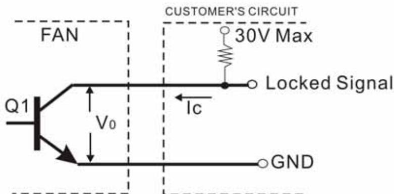
\*Transistor Q1 at "ON" position
