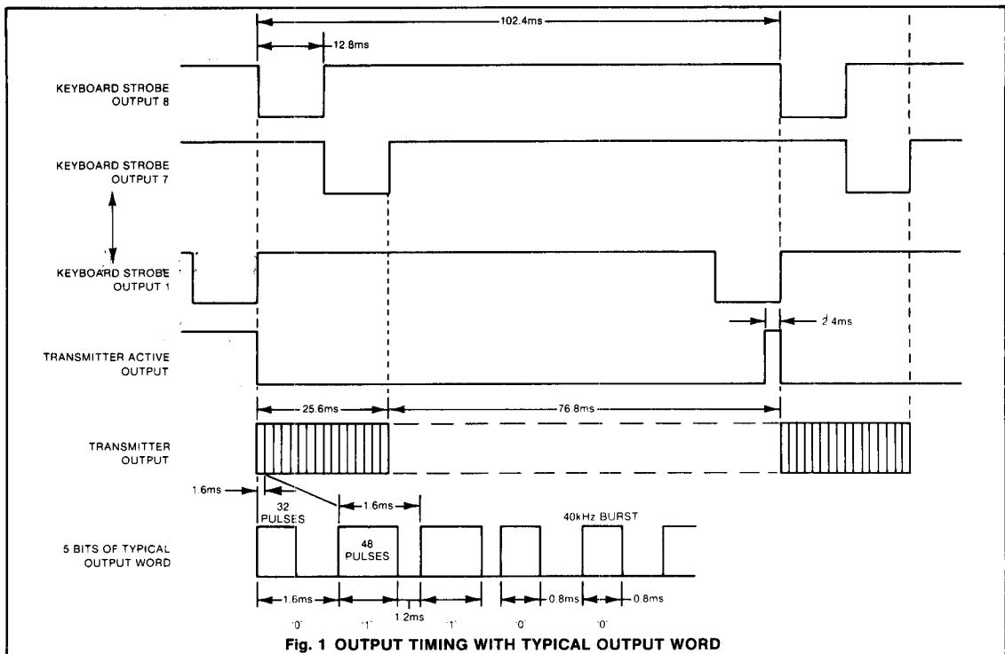
Fig. 1 OUTPUT TIMING WITH TYPICAL OUTPUT WORD
