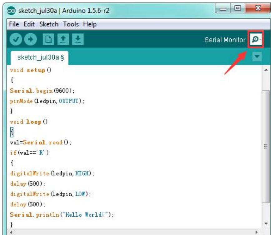
Then set the baud rate as 9600, enter an "R" and click Send, you should see the RX led on the board blink once, and then D13 led blink once, finally "Hello World!" is showed on the monitor, the TX led blink once.
