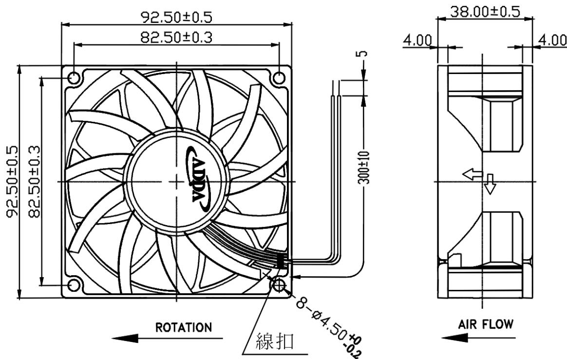
LEAD WIRES : UL 1007, AWG24 , L = 300±10 mm
