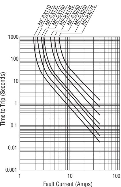
The Time to Trip curves represent typical performance of a device in a simulated application environment. Actual performance in specific customer applications may differ from these values due to the influence of other variables.
