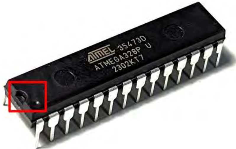
Figure 11: ATmega328P Pin 1 marking (dot indent) and half-circle marking (half-circle indent).
