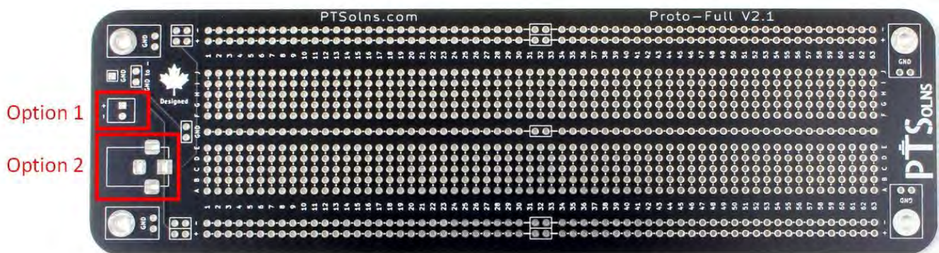
Figure 1: Two power input options for the Proto-Full.
