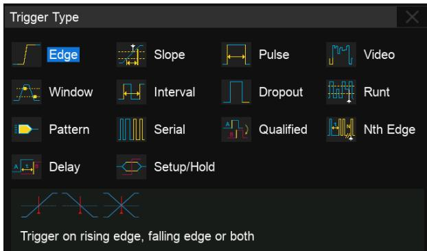
Edge, Slope, Pulse width, Video, Window, Runt, Interval, Dropout, Pattern, Qualified, Nth edge, Delay, Setup/Hold time, and Serial trigger.
