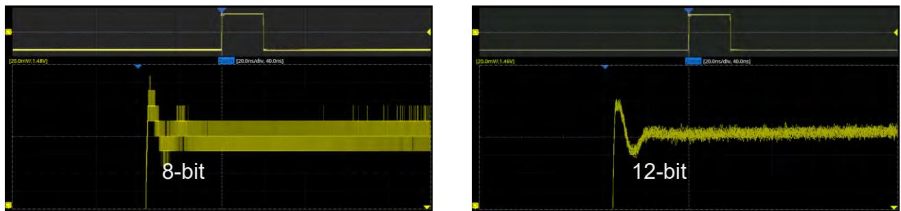
Vertical & Horizontal Zoom along with a large memory depth make the most out of 12-bit ADC resolution. Engineers can observe waveform overall and details simultaneously.
