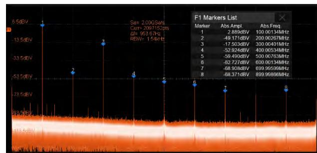
Hardware-accelerated FFT supports up to 2 Mpts operation. This provides high-frequency resolution with a fast refresh rate. The FFT function also supports a variety of window functions so that it can adapt to different spectrum measurement needs. Three modes (Normal, Average, and Max hold) can satisfy different requirements for observing the power spectrum. Auto peak detection and markers are supported.
