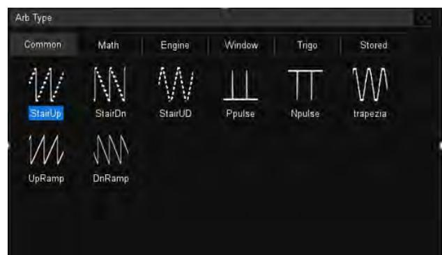
The USB waveform generator can output waveforms with up to 25 MHz frequency and  $\pm 3$  V amplitude. Six basic waveforms together with multiple types of predefined waveforms and as user-defined arbitrary waveforms are supported.
