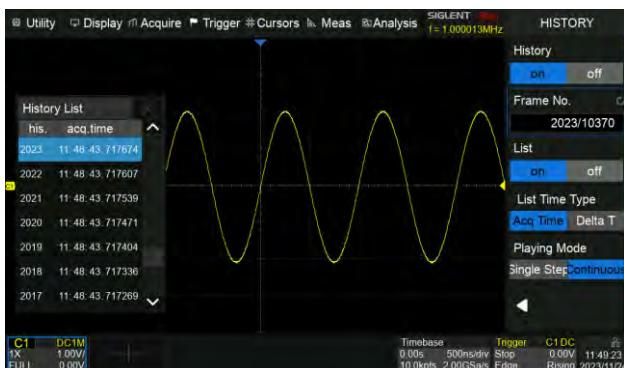
History function can record up to 80,000 frames of waveforms. The recording is executed automatically so that the customer can playback the history waveforms at any time to observe unusual events and quickly locate the area of interest using the cursors or measurements.
